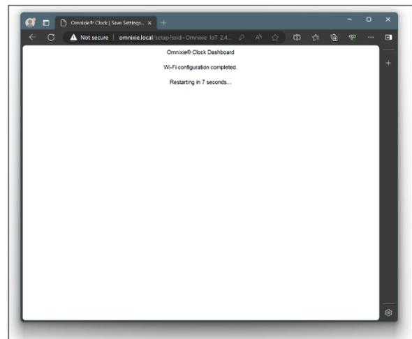
After the WiFi configuration is completed, The Omnixie Will reboot and connect to the WiFi automatically. If the connection is successful, the WiFi status indicator will light **yellow** or **green**. If WiFi status indicator still red after rebooting, it indicates that the WiFi password just entered is incorrect, please select again to make settings.
