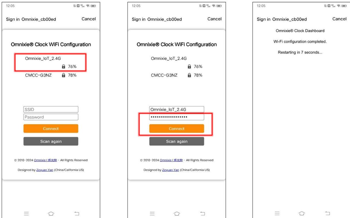
After the WiFi configuration is completed, The Omnixie will reboot and connect to the WiFi automatically. If the connection is successful, the WiFi status indicator will light **yellow** or **green**. If WiFi status indicator still red after rebooting, it indicates that the WiFi password just entered is incorrect, please select again to make settings.
